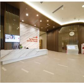
Taralay Impression Comfort is an acoustic solution with Very High Density (VHD) foam backing reinforced with glass fibre and has a printed design protected by a transparent wear layer 0.65mm thick. It offers 19dB sound insulation and indentation resistance of 0.08mm.
