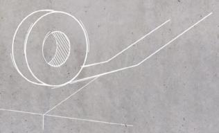
$38.2 \pm \text{Cut}$  masking tape at the seam using a knife with a new blade.
