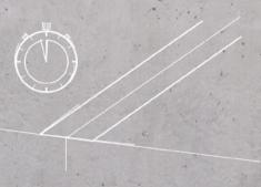
3B.5- Remove the masking tape which will also remove the excess seam sealer.
