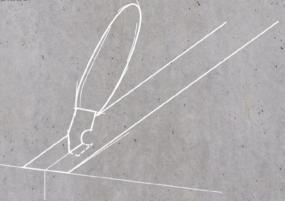
3B.3 - Insert the needle into the seam pulling towards you and slowly apply the liquid until it penetrates the seam and beads up onto the masking tape.
